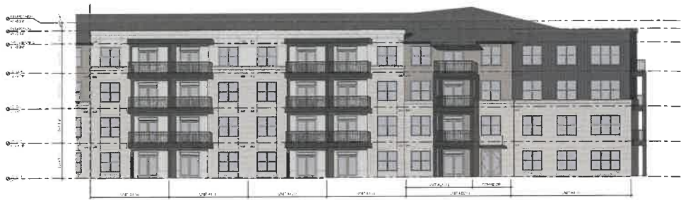
BLOCK 01 - EAST ELEVATION - PART A 1/8" = 1'-0"
